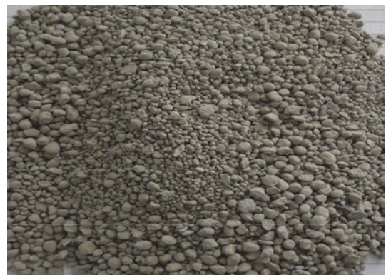
Figure 1. Fly ash aggregate (FAA)
