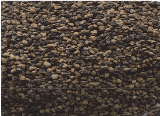
Figure 2. Light expanded clay aggregate (LECA)
